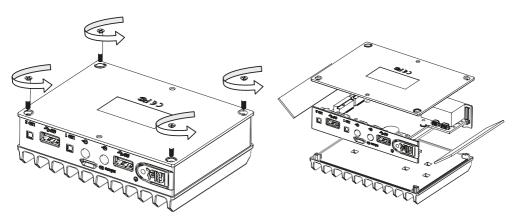
Open the bottom cover by unscrewing 4 philips-head screws.
