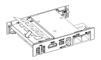
The RAM is located under the top cover of the Pokini F2.
