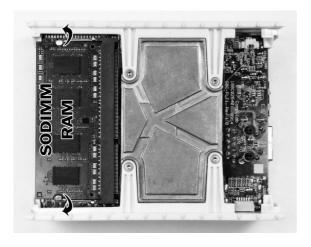
4. SODIMM which is located at the top side of the motherboard is now accessible for installation/replacement
