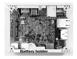
mSATA, SIM socket, miniPCle and battery which are located at the bottom side of the motherboard are now accessible for installation/ replacement.
