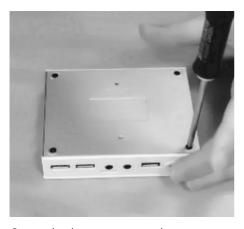
Open the bottom cover by unscrewing 4 philips-head screws.
